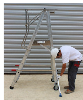
Installing the stabilizers
